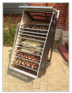
It is made from marine ply for the three sides. The runners just alu angle. The frame is at about 60 degrees.
